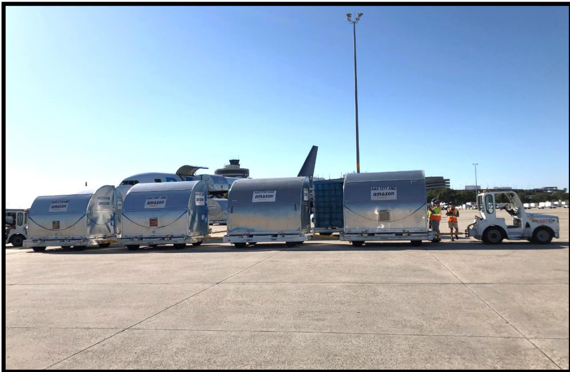
No more than four ULDs can be towed at a time
