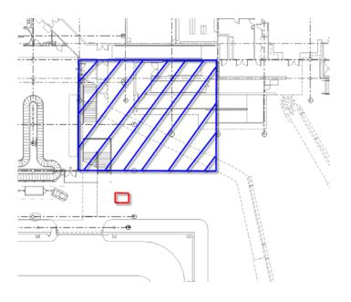
One (1) 275 gallon Grease Trap just outside of tug tunnel. Serves Illy. Located to avoid proposed future expansion of A/S-F Ramp Level.
