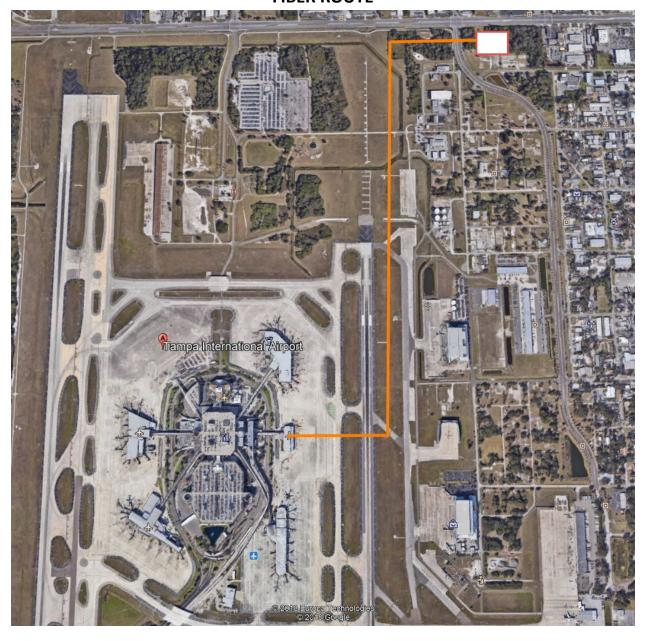
Above is a possible fiber route from the head end building site, west, then south in-between 1R/19L and taxiway "E" then under the runway, through the grass, under the apron and into A-Sort. From there, into the terminal building and into the Communications Equipment Room (whether it's 4<sup>th</sup> floor A-core or elsewhere). The fiber route would need to be reviewed by all interested parties, utility locates and perhaps GPR to see what might lay below the surface.
