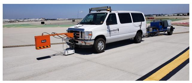
Figure 14 ARA HWD integrated with a GPR
