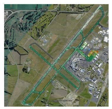
Figure 10 Detailed Distress Locations and PCI Scores
