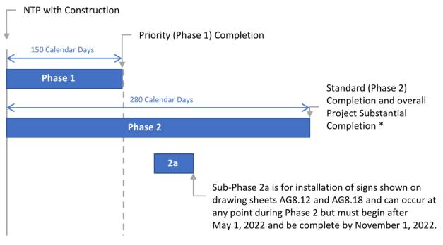
**Schematic Construction Phasing Diagram**
